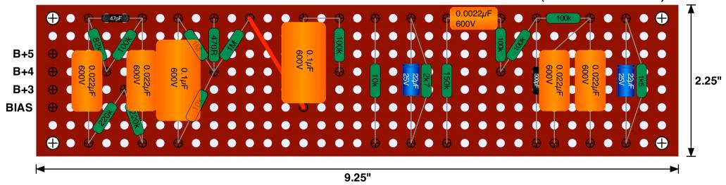
All parts and boards are to scale and can be used as a template for DIY.
